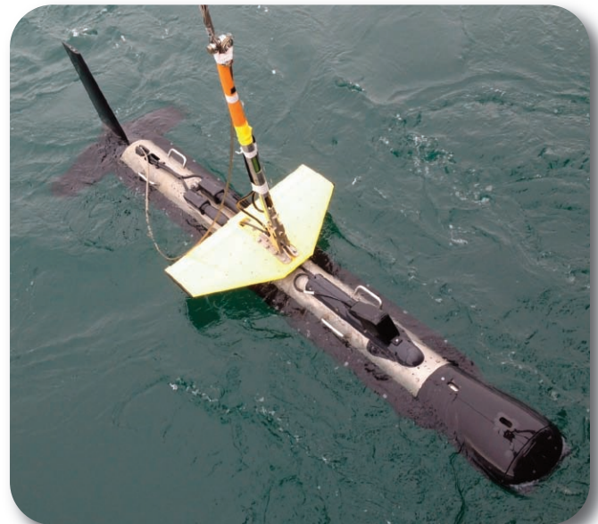
Klein System 5900 with optional K-Wing IV and Gap Filler Sonar
